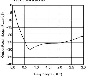
RFC-RF1/RF2 UNUSED PORT RETURN LOSS vs. FREQUENCY
